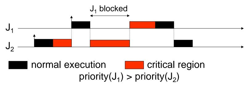
Here: Blocking time equal to length of critical section.
