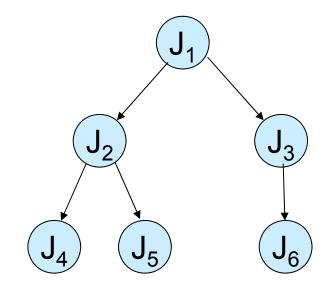
$J_1 \langle J_2 : J_1 \text{ is a predecessor of } J_2 \rightarrow J_1 \text{ must be executed before } J_2$
