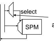
Selection is by an appropriate address decoder (simple!)
