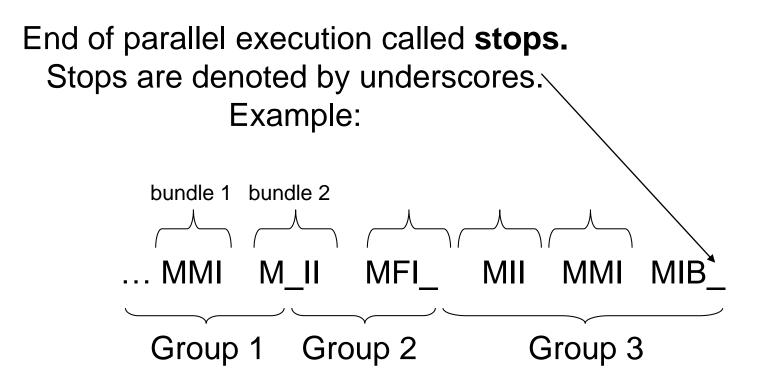
Very restricted placement of stops within bundle. Parallel execution within groups possible. Parallel execution can span several bundles
