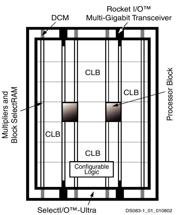
Virtex II Pro Devices include up to 4 PowerPC processor cores
