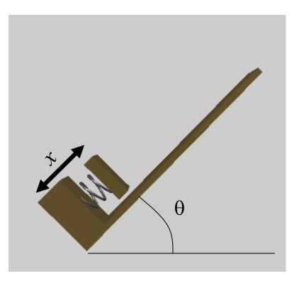
Component of gravitational force in the direction of the accelerometer axis must equal the spring force:
