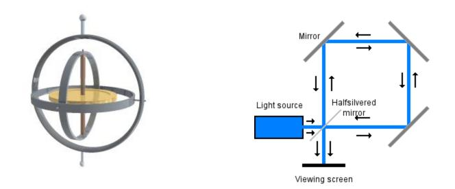
Optical gyros: Leverage the Sagnac effect, where a laser light is sent around a loop in opposite directions and the interference is measured. When the loop is rotating, the distance the light travels in one direction is smaller than the distance in the other. This shows up as a change in the interference.
