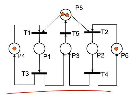
$$\underline{N^{T} c_{R}} = \mathbf{0}, \text{ with } \underline{N^{T}} = \begin{bmatrix} P1 & P2 & P3 & P4 & P5 & P6 \\ T1 & 7 & \phi & \phi & -7 & -7 & \phi \\ T2 & \phi & 7 & \phi & 0 & -7 & -7 \\ T3 & -7 & \phi & 7 & 7 & 0 & \phi & 7 \\ T4 & \phi & -7 & 7 & 0 & \phi & 7 \\ T5 & \phi & \phi & -1 & \phi & 7 & \phi \\ \end{bmatrix}$$
