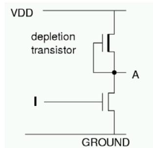
Depletion transistor (resistor) contributes a weak value to be considered in the #-operation for signal A
