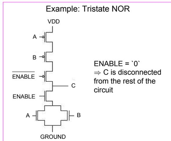
We introduce signal value 'Z', meaning „high impedance“
