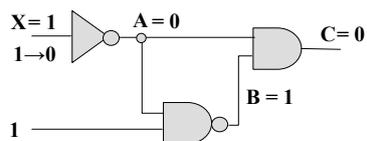
Simulation time does not proceed due to delta delays!
