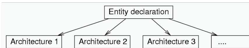
Each architecture includes a model of the entity. By default, the most recently analyzed architecture is used. The use of another architecture can be requested in a **configuration**.
