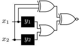
**Fig. 1.** Example of a partial equivalence checking (PEC) problem. A partial design, consisting here of the two black boxes and the OR gate, is compared to the reference circuit above, here consisting of a single XOR gate. The output of the complete circuit is 1 iff the completion of the partial design and the reference circuit compute the same result.
