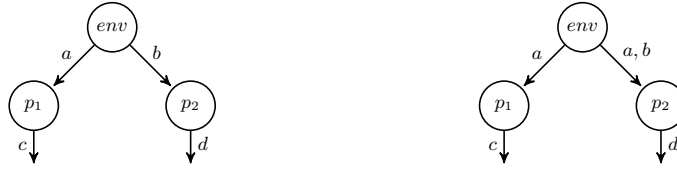
(a) An architecture of two processes that specify process p_1 to produce c from a and p_2 to produce d from b . (b) The same architecture as on the left, where only the inputs of process p_2 are changed to a and b .
