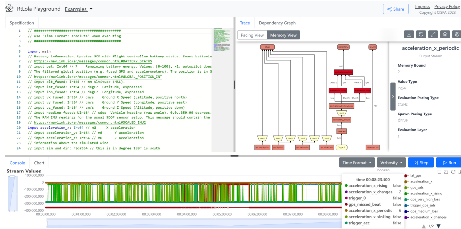
Fig. 2: Screenshot of the RTLola playground. The left panel contains the specification editor, the right panel the dependency graph and the trace editor, and the bottom panel contains the output of the interpreter as the CLI output and a plot.
