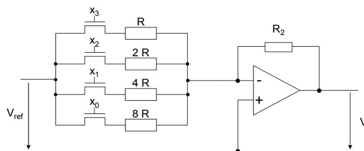
$$V = -V_{\text{ref}} \cdot \frac{R_2}{R_T} = -V_{\text{ref}} \cdot \frac{R_2}{2^{4-i} R} (< \times >)$$
