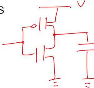
Charge of capacitor:  $q = V_{dd} \cdot C$
