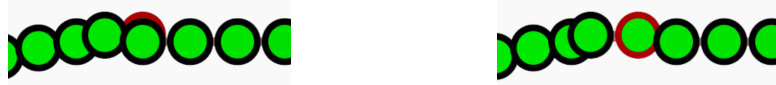
Fig. 4: On the left side, one marker with irrelevant information covers a critical marker, whereas the monitor on the right encodes a form of priority.
